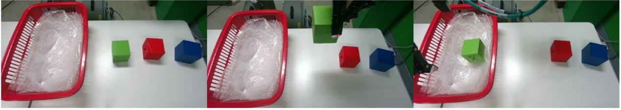
Fig. 2. Demonstration of a pick-and-place task using a physical robot and our planning pipeline. Initially, three RGB-colored blocks are placed in a row next to the basket (leftmost image). The goal is to identify the closest block to the basket and drop it into the basket (rightmost image).
