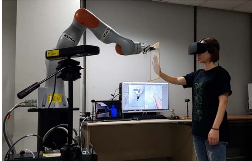
Figure III-2. An encountered-type haptic tracking system with fixed RGBD camera and HMD tracking system
