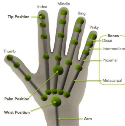
Figure 12: Leap Motion skeletal hand taxonomy Figure is taken from Leap Motion official blog [54]
