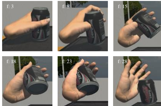
Figure 17: Grasping sequence without proxy hand, showing penetrations Captured at different frames showing holding, moving and releasing the object (top left to bottom right)
