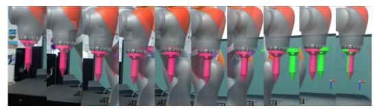
Figure 17. AR simulation of the path between the start pose and goal pose of the tool
